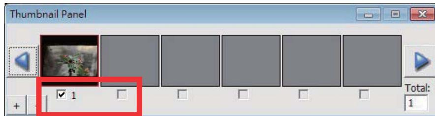
When scanning more than 6 frames (6 at a time are viewable in the thumbnail panel) you may scroll to view more by clicking on the right arrow button. the left / right arrow buttons allow you to scroll through pre-scanned images with ease. this model scanner is capable of scanning an entire roll of (uncut) film up to 40 frames
