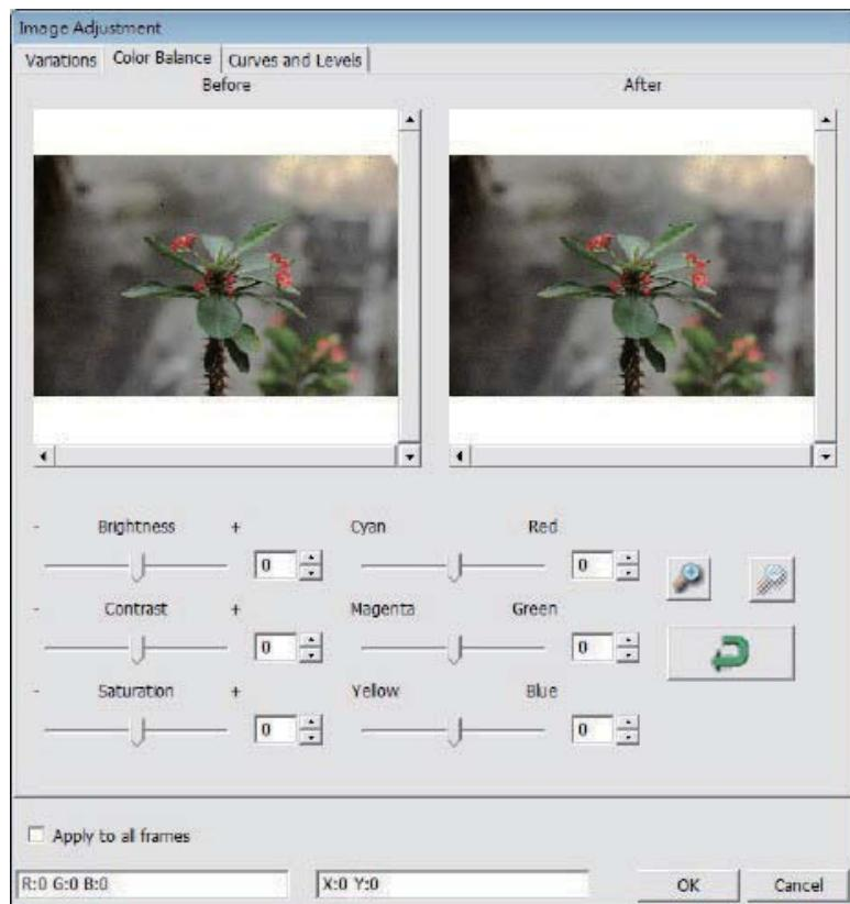
**Example:** if a previewed image appears too dark, use the "Brightness" slider in the "Color Balance" window to adjust the image by selecting the slider in the center and moving it to the right. the image's "after" view becomes lighter. select "ok" to accept the changes which will be sent to the scanning hardware. this can also be used to adjust each of the functions in "Color Balance" by contrast, saturation and specific color ranges of cyan, magenta and yellow.
